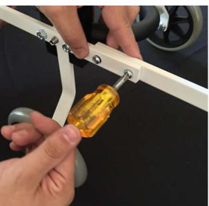
3) Slide front wheel blades into the front blocks, and set initial height so the front is level with the back. Tighten the temporary set screw on the outside. **Note:** This is a temporary screw. Once the correct height is determined, mark the height on the wheel blades and remove the temporary height adjustment screw. Tighten the inside set screw in the block, to hold the wheel blades in place long-term.
