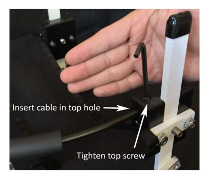
2) Loop the cable around, forming a circle. Push the other end of the cable through the top front hole of the block. Push the cable through until each end of the foam is touching the block. Tighten the front set screw on the top of the block. **Note:** Do not over tighten the set screws holding the cable. They just need to be tightened until the screw stops turning.
